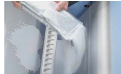
1 Pour the hot melt powder into the powder shaking system. The maximum capacity is 1.5kg.
