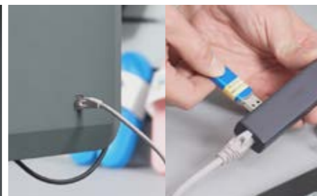
30 Connect the printer and computer with a network cable. Plug in the dongle.
