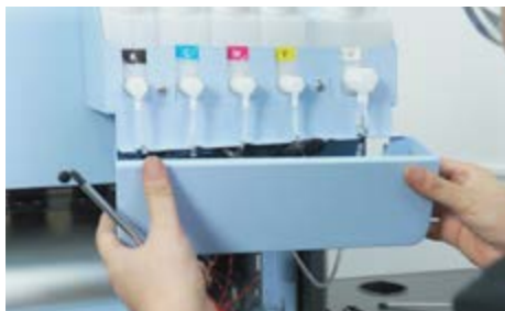
22 Install the cover back in place.
