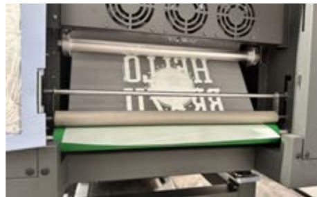
8 Lower the rod to secure the film.
