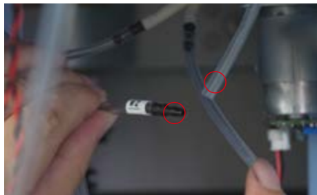
19 Connect W2 to the reflux tube.
