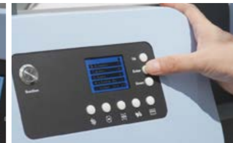
5 Activate the powder shaking and drying system.
