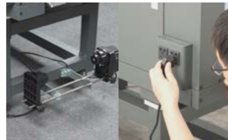
25 Install the auto film take-up system and connect its power cable.
