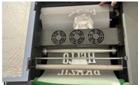
7 Wrap the printed film as shown above.
