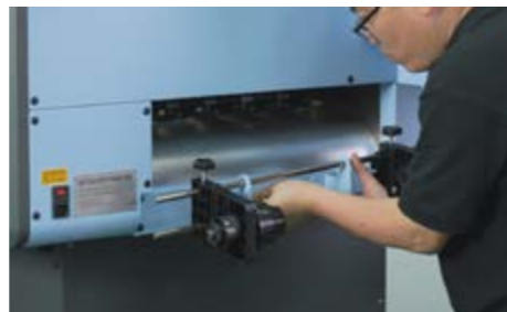
24 Install the film roll holder onto the back of the printer.
