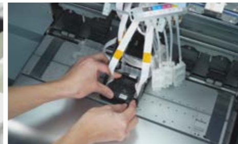
33 Install the printhead and perform printhead calibration.
