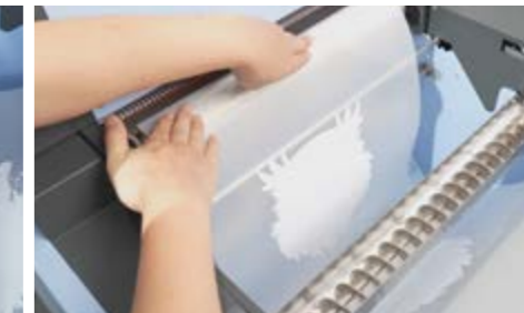
3 Once the printed film reaches a suitable length, pick up the end of the film and extend it to the oven.
