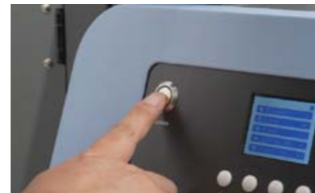
4 Press the "Suction" button, which will securely attach the film to the platform.
