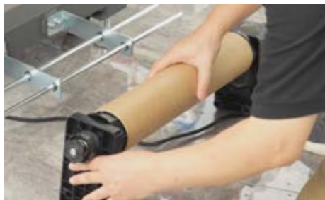
10 Wait until the printed film reaches a length suitable for take-up. Then, install the roll core onto the auto film take-up system and adjust its position as needed.
