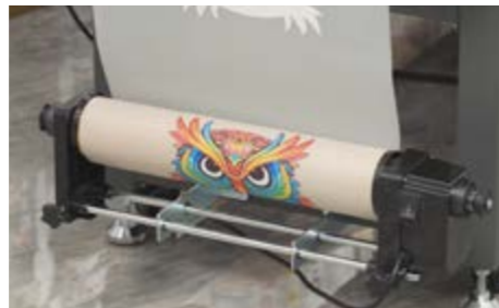
11 Secure the film onto the core, then activate the device and adjust the tension of the damper.
